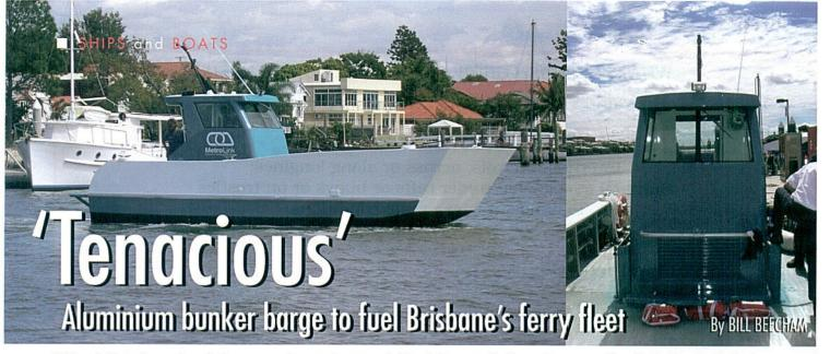
The 9.5-metre aluminium work barge/bunker barge 'Tenacious' is the latest addition to the fleet of vessels operated by Metrolink Queensland.
